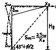
Fig. 4-1 Estimation model of triangular ground movement
