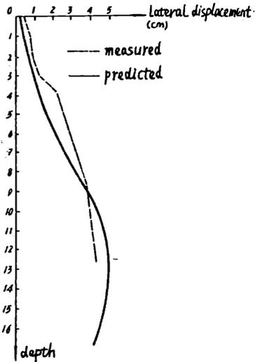
Fig.5-8 Curves of lateral displacements of the diaphragm wall
