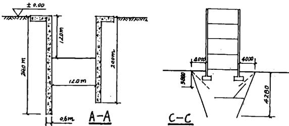
Fig. 5-2 Fig. 5-3 Cross-sections of excavation and building
