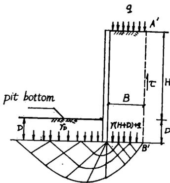
Fig. 2-1 Slip curve considering  $C$  and  $\phi$  simultaneously
