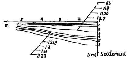
Fig. 5-6 Curve of building settlement (Northern side)
