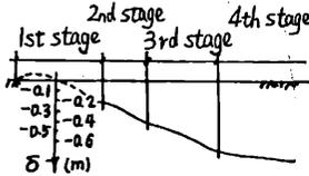
Fig. 4-4 Curve of settlement with time
