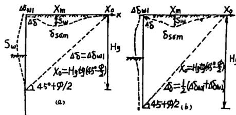
Fig.4-2 (a) (b) Estimation model of parabola ground settlement
