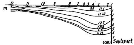
Fig. 5-5 Curve of ground settlement
