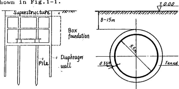
Fig. 1-1 Cross-section of Xingzha Road Station and tunnel
