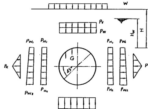
Fig.3-2 Design loads on a shield tunnel
