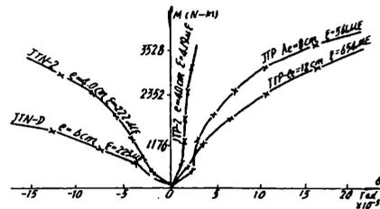
Fig. 3-7  $M-\theta$  Curve of joint when accentrally loaded
