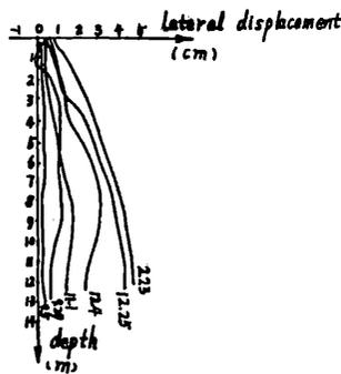
Fig. 5-4 Lateral movement curve of the diaphragm wall
