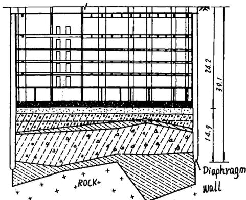
Fig. 1-2 Six-storey basement of New Century Mansion
