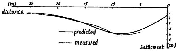
Fig. 5-7 Curves of ground settlements
