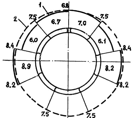
Fig.3 Comparison of the measured (1) and the designed (2) contact stresses ( $1 \cdot 10^2 \text{ MPa}$ ) on subway tunnel lining
