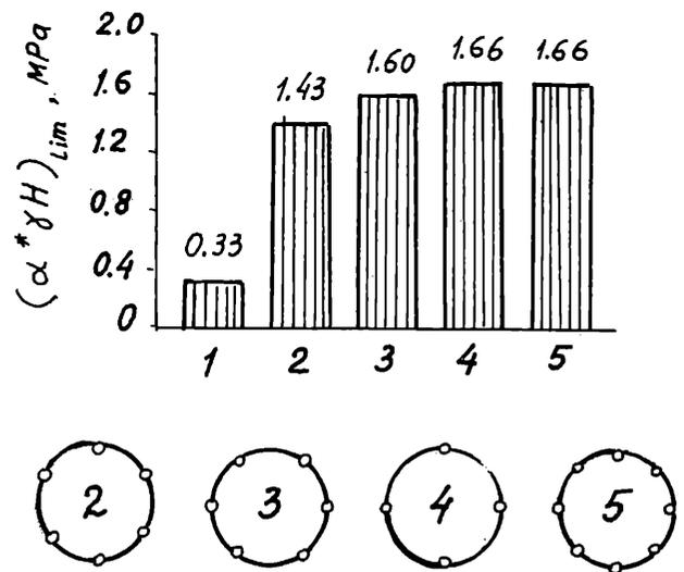
Fig.5 Bearing capacity of the tunnel lining depending on its construction
