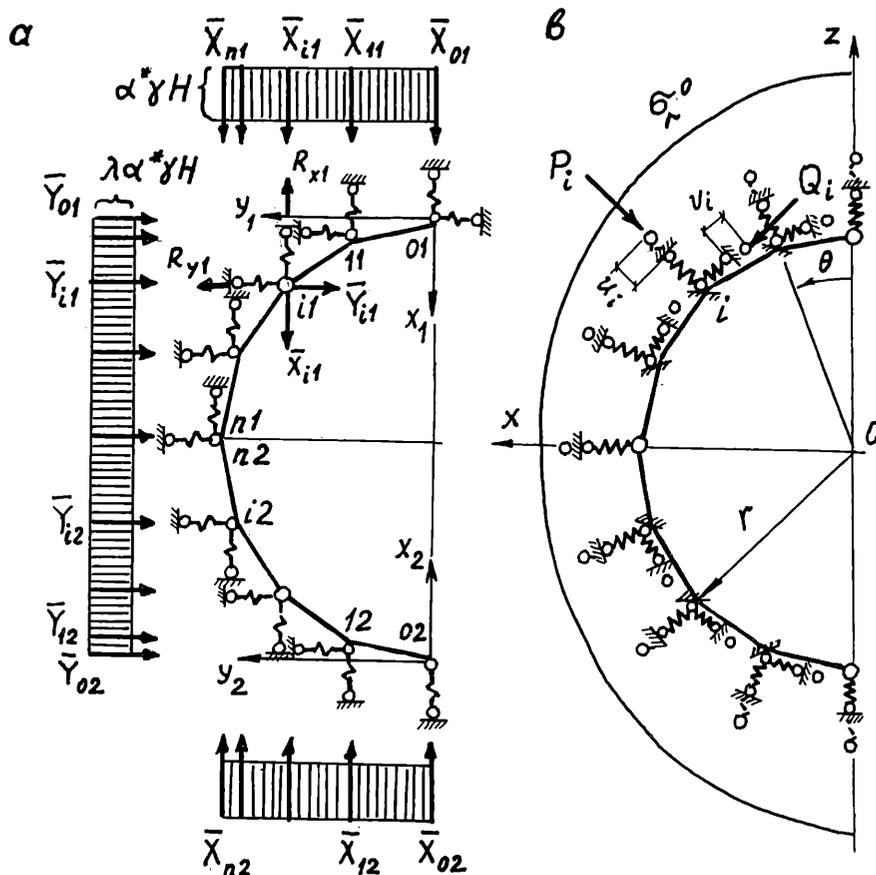
Fig.1 Design scheme of pre-fabricated lining
