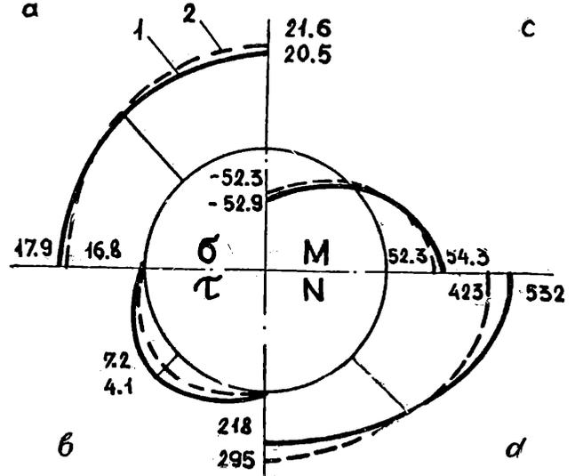
Fig.2 Comparison of design values (2) the  $\sigma$  and  $\tau$  contact stresses ( $1 \cdot 10^2 \text{ MPa}$ ), the  $M$  and  $N$  internal forces with those obtained from the accurate solution of elasticity theory problem (1).
