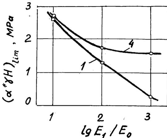
Fig.6 Correlation between bearing capacity of the monolithic (1) and prefabricated linings (2) and the  $E_1/E_2$  Ratio of the  $E_1$  reinforced concrete and  $E_2$  ground deformation modulae
