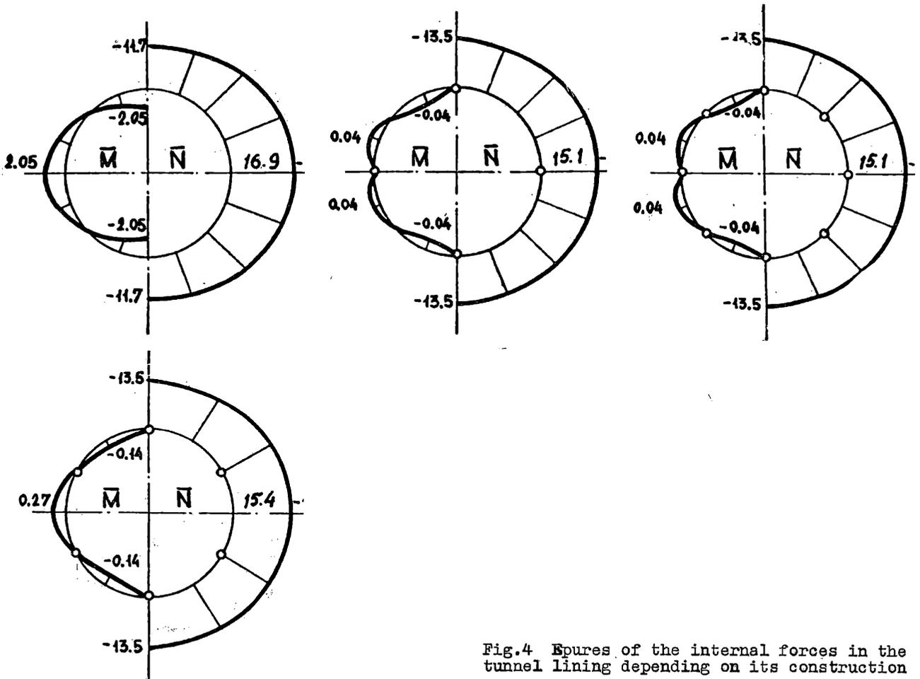
Fig.4 Epures of the internal forces in the tunnel lining depending on its construction
