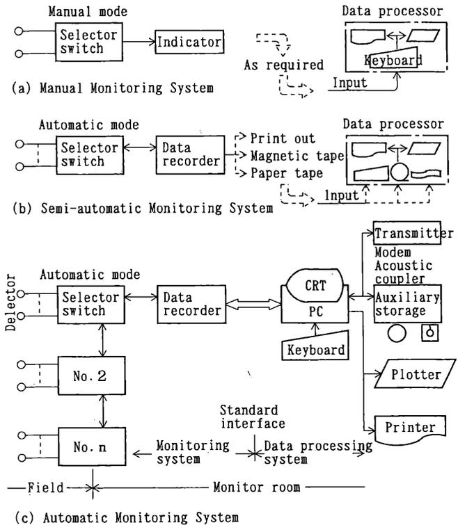
Figure 1. Diagrams for field monitoring system
