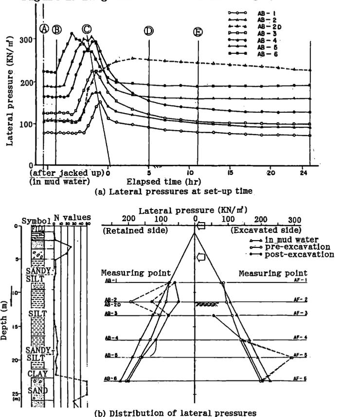
Figure 2. Lateral pressure at set-up time and lateral pressure distribution after excavation (Kanatani et al., 1980)
