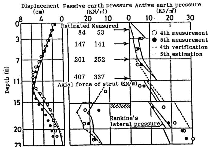
Figure 6. Prediction based on lateral pressures obtained by back analysis (Maruoka et al, 1984)
