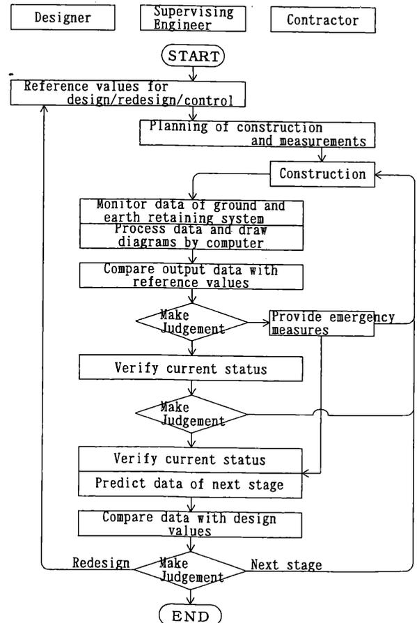
Figure 4. Flow chart of construction control by monitoring (observational procedures)
