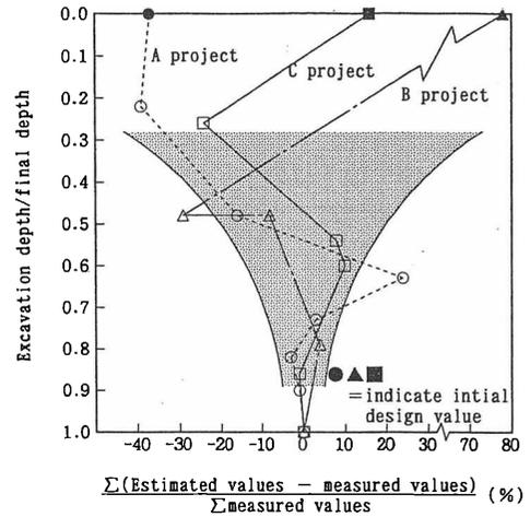
Figure 5. Comparison between estimated and measured values (Tominaga et al, 1977)
