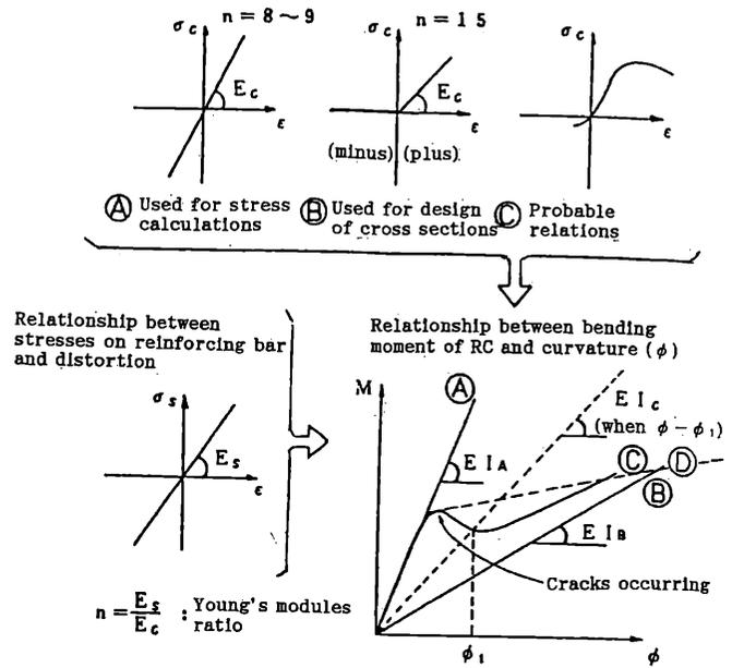
Figure 3. Assumed flexural rigidity of RC diaphragm wall (Hayakawa and Honda, 1984)
