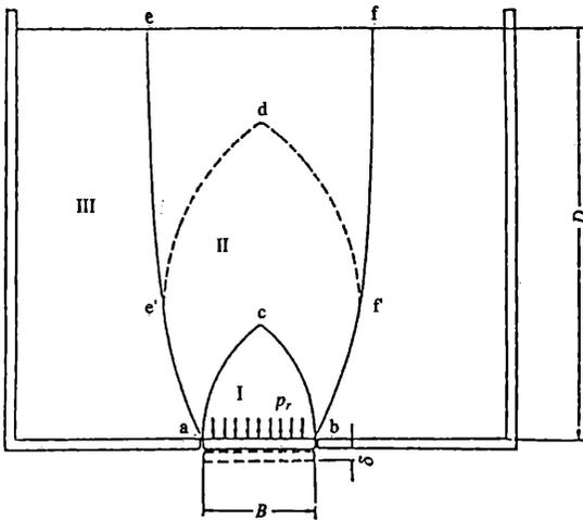
Fig. 4 Different movement areas of sand layer caused by trap door (Murayama, S., 1970)
