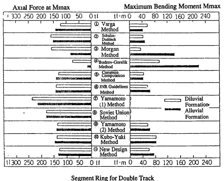
Fig. 8 Comparison of computed sectional force (Hanya et al. 1987)
