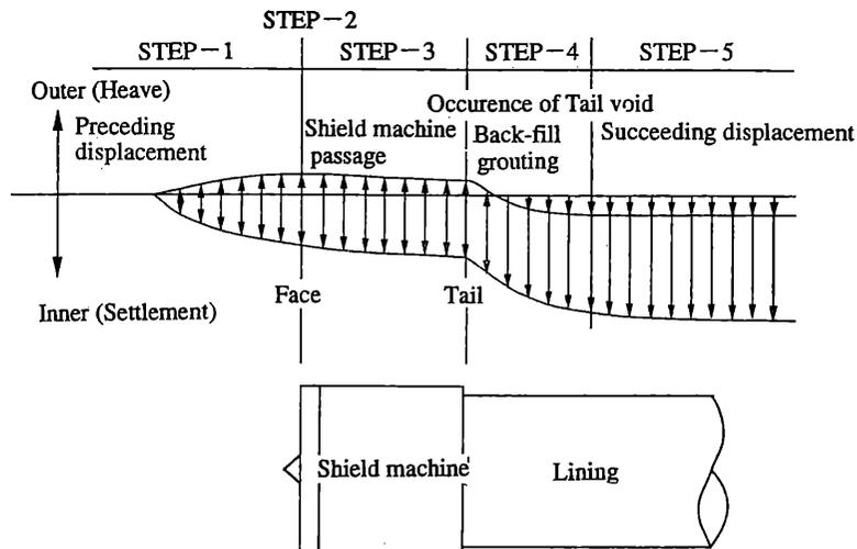
Fig. 1 Advancement of shield machine and ground displacement
