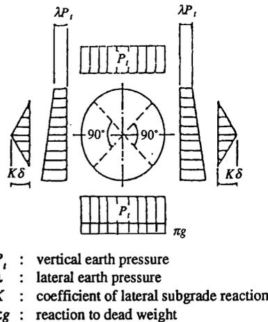
Fig. 5 Assumption of subgrade reaction based on common model
