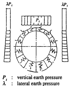
Fig. 6 Assumption of subgrade reaction based on spring bedding model
