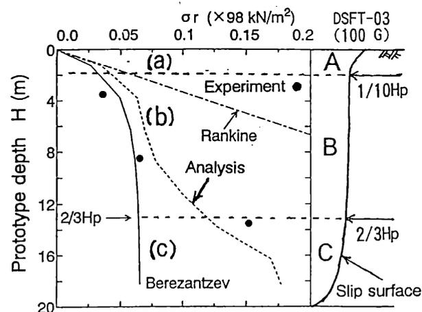
Figure 8 Earth pressure on shaft wall (Fujii et al.)
