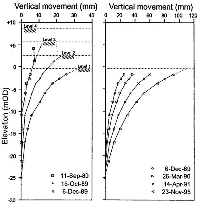
Figure 5 Vertical movements at various stages (Nash et al.)
