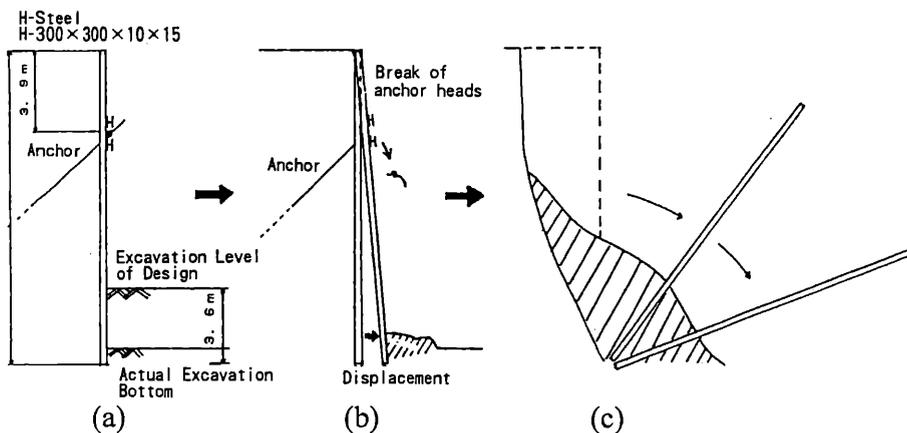
Figure 2. Estimated failure mechanism (Toyosawa et al.)
