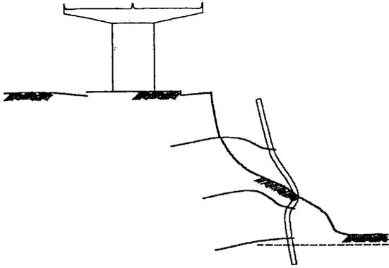
Figure 1. Section after failure. (Maffei et al.)
