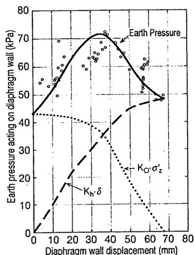
Figure 4. Change in earth pressure with diaphragm wall displacement (Tamano et al.)
