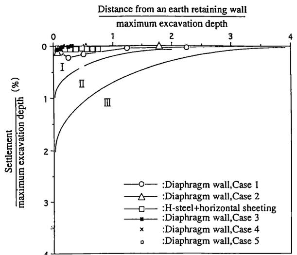
Figure 15. Peripheral ground surface settlement during shaft excavation
