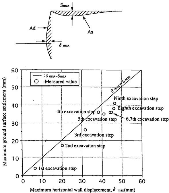
Figure 16. Relationship between maximum horizontal wall displacement and maximum ground surface settlement
