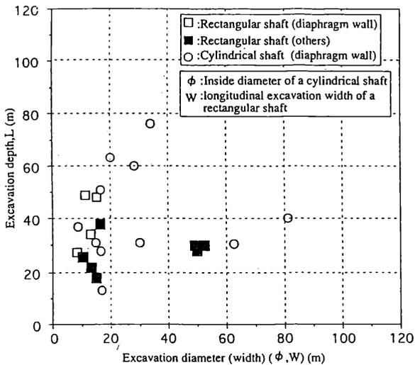
Figure 2. Relationship between excavation width (diameter) and excavation depth (L)
