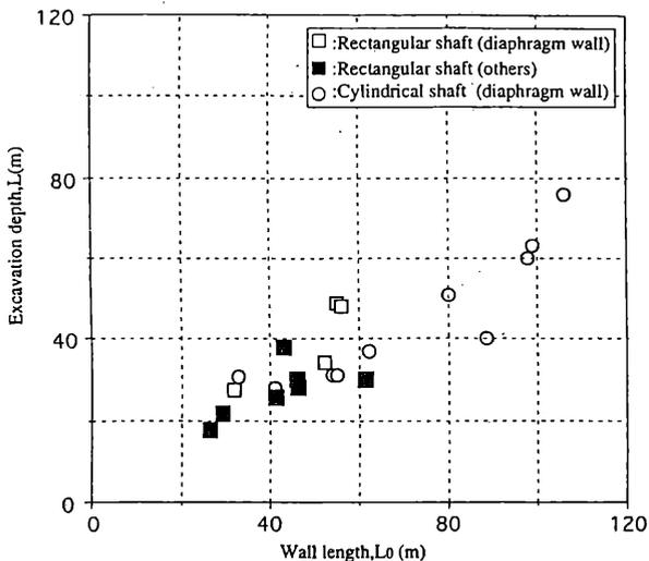
Figure 3. Relationship between wall length ( $L_0$ ) and excavation depth (L)
