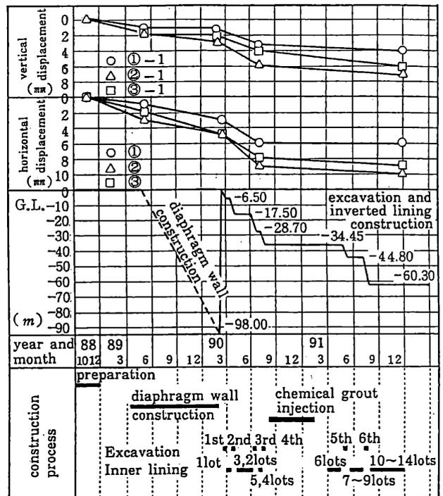
Figure 12. Construction progress records and changes in ground surface displacement with the passage of time<sup>1)</sup>
