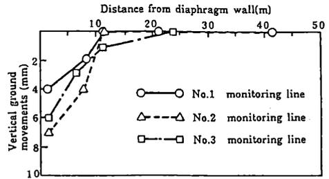
Figure 11. Ground surface settlement around the shaft after the completion of excavation
