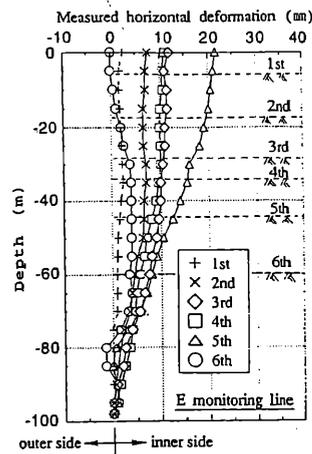
Figure 8. Changes in measured horizontal wall displacement with depth<sup>1)</sup>
