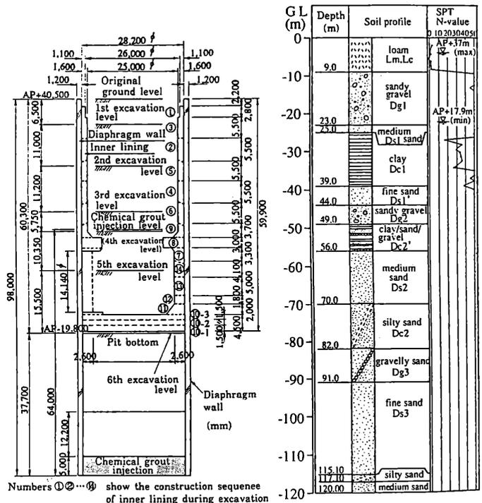
Figure 5. Longitudinal section of the shaft<sup>1)</sup>
