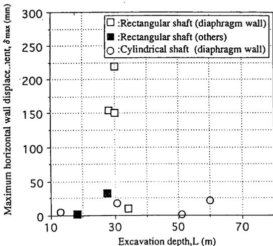
Figure 13. Relationship between excavation depth and maximum horizontal wall displacement (shaft)
