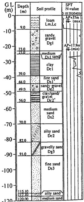
Figure 6. Geological profile and soil conditions near the shaft
