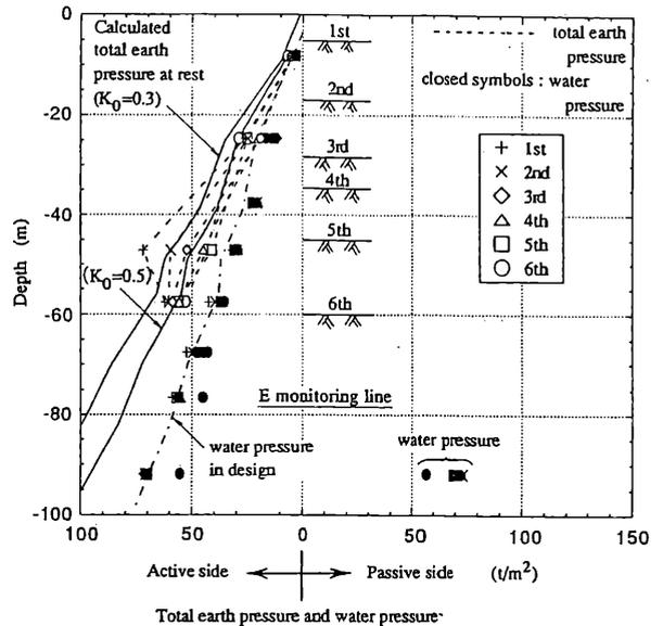
Figure 7. Lateral pressure and hydrostatic pressure measured (on measuring line E)<sup>1)</sup>
