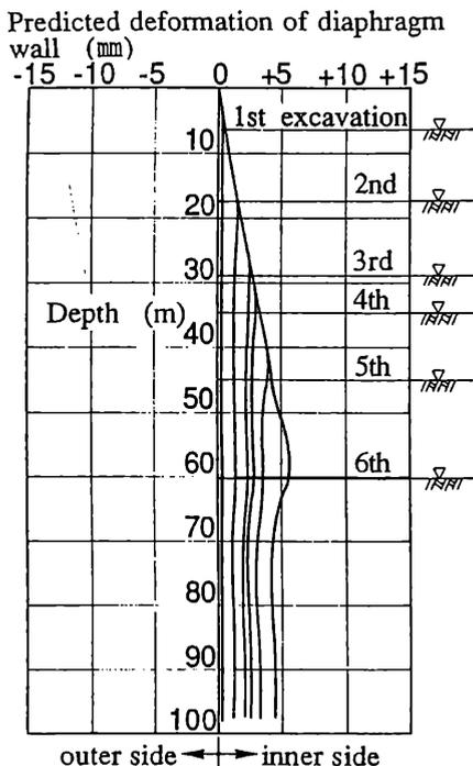
Figure 10. Predicted displacement of the wall<sup>1)</sup>
