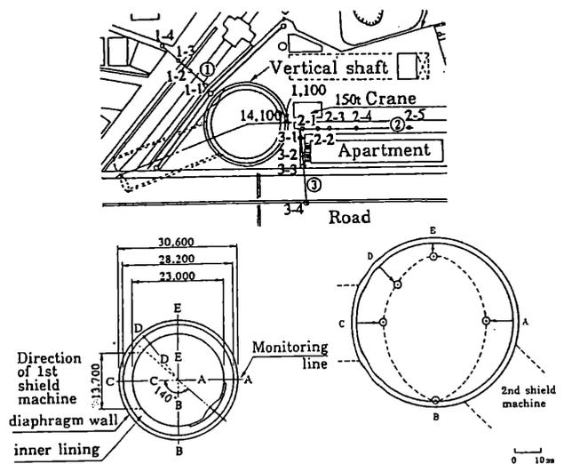
Figure 9. Wall deformation at ground surface on measuring lines
