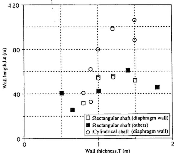
Figure 4. Relationship between wall thickness and wall length ( $L_0$ )
