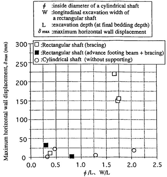
Figure 14. Relationship between aspect ratio and maximum horizontal wall displacement by shaft shape
