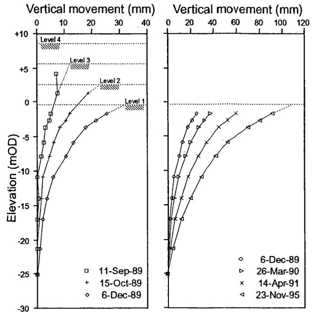
Figure 4. Movements at various dates - a) after each stage of excavation, and b) since end of excavation.
