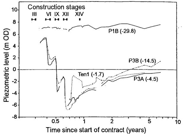
Figure 6. Piezometric levels vs time.
