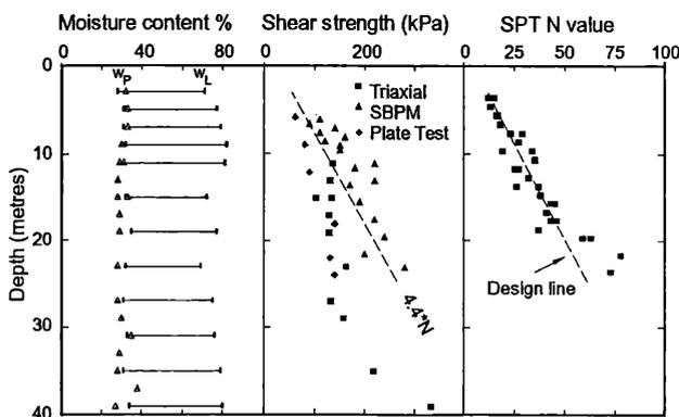
Figure 2. Geotechnical profile
