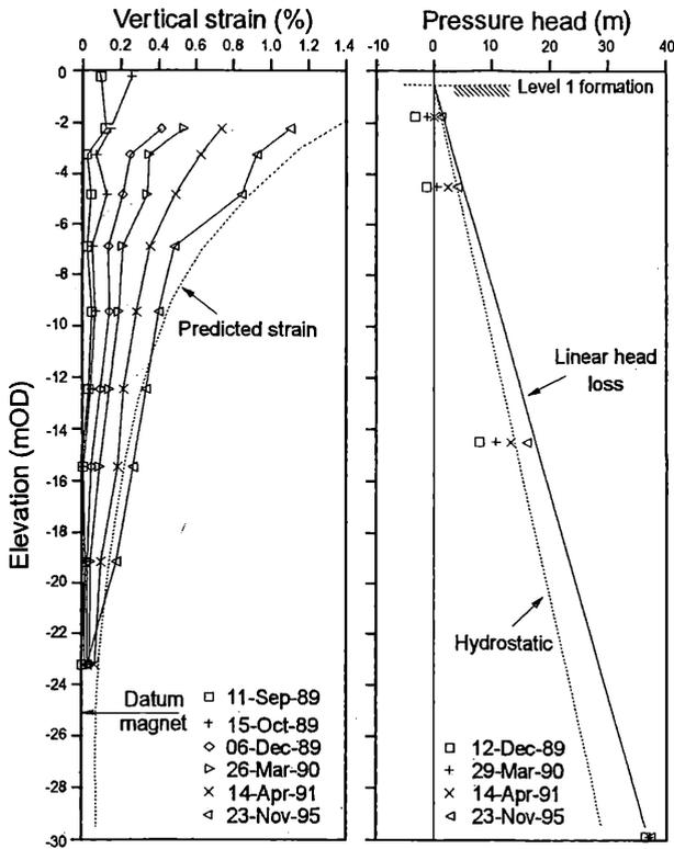
Figure 5. a) Vertical strains, and b) Pressure heads at various dates.
