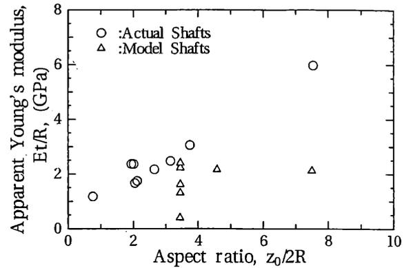
Fig. 2: Comparison between model shafts and actual shafts
