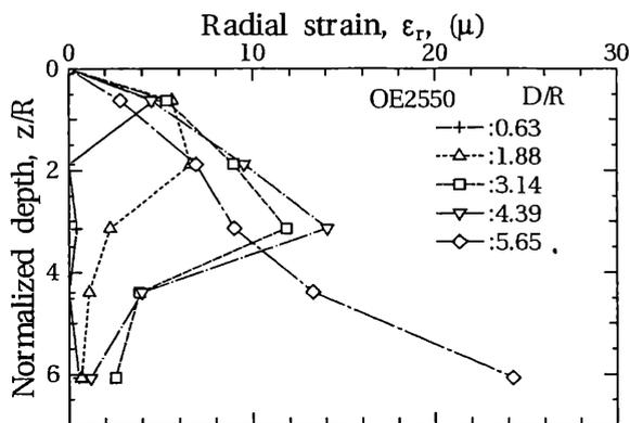
Fig. 4: Changes of the distribution of radial strain  $\epsilon_r$  during an excavation process
