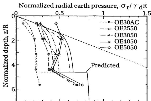
Fig. 11: Predicted and measured distributions of  $\sigma_r / \gamma_d R$
