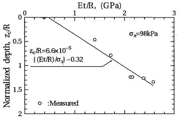
Fig. 10: Changeover depth  $z_c$  versus apparent Young's modulus  $Et/R$
