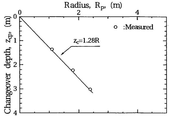
Fig. 9: Changeover depth  $z_c$  versus radius of shaft  $R$
