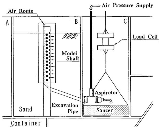
Fig. 3: Soil container and vacuum excavator
