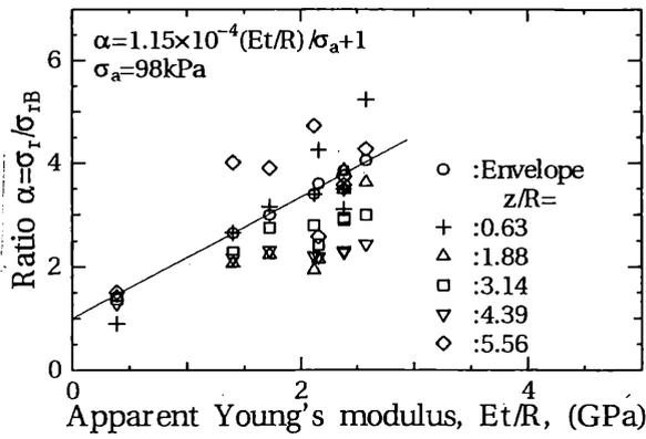
Fig. 7: Ratio  $\alpha$  versus apparent Young's modulus
