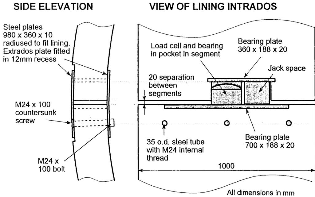
Figure 2 - Details of load cell pocket.
