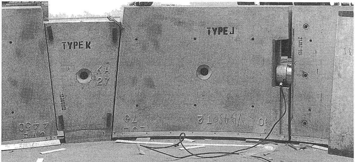
Figure 5 - Trial build of expanded ring showing load cell recess.
