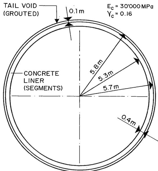
Fig. 10 Boundary conditions for design
