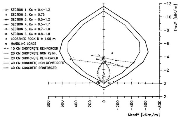
Fig. 9 Forces obtained from verification
