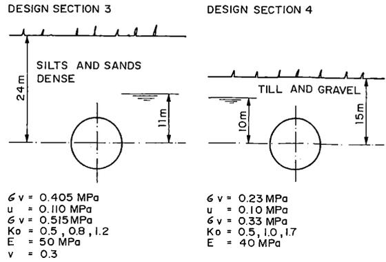
Fig. 5 Design eastern soil section
