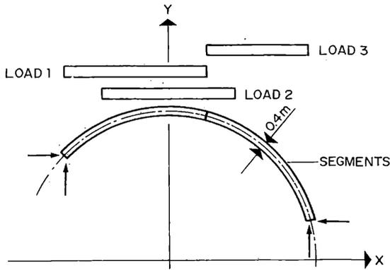
Fig. 7 Loosening Loads on Segments
