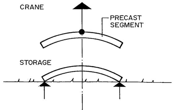
Fig. 6 Handling Loads on segments
