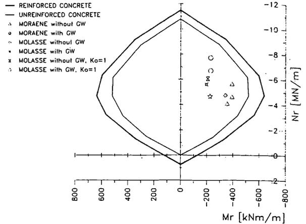
Fig. 8 Interaction diagram with contractor's results
