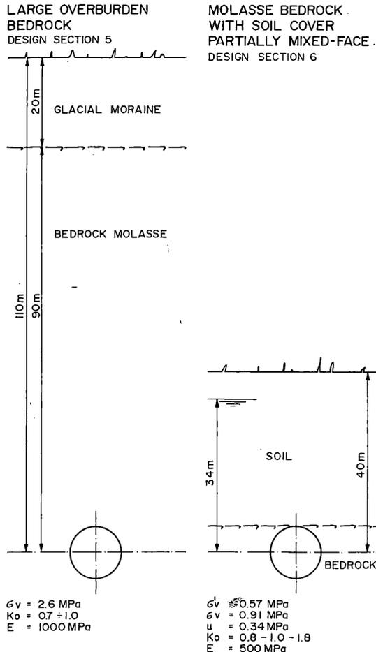
Fig. 4 Design section in bedrock
