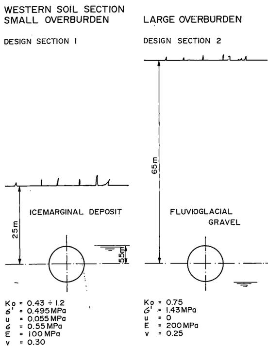
Fig. 3 Western soil section design conditions
