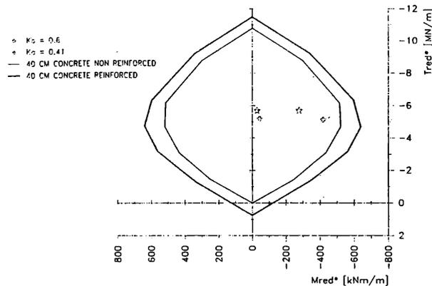
Fig. 11 Interaction diagram with effect of reduced bending stiffness
