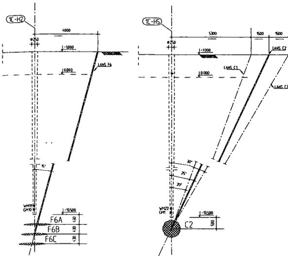
Figure 7. Compensation grouting; compaction grouting (left) and fracturing (right).
