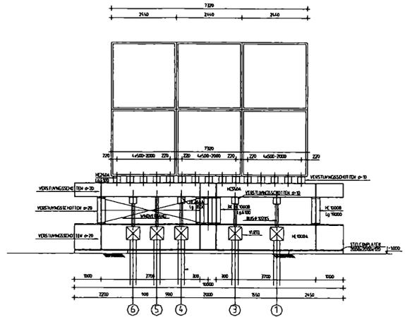
Figure 1. Cross Section of the Ballast Frame.
