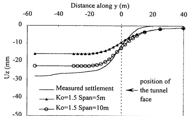
Figure 4. Longitudinal ground surface settlement along the centreline of the tunnel
