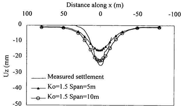
Figure 3. Transverse ground surface settlement on the completion of the excavation.
