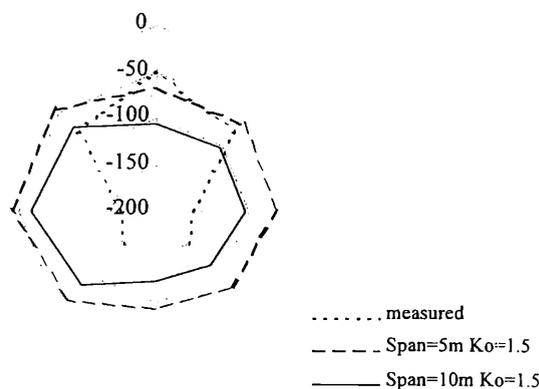
Figure 6. Excess pore pressure at the transverse section.
