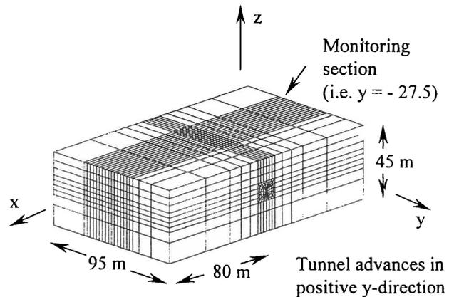
Figure 2. 3D Finite element mesh.
