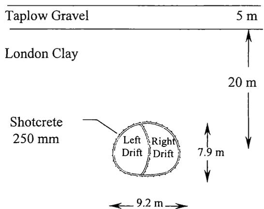
Figure 1. Tunnel geometry and the modelled soil profile.
