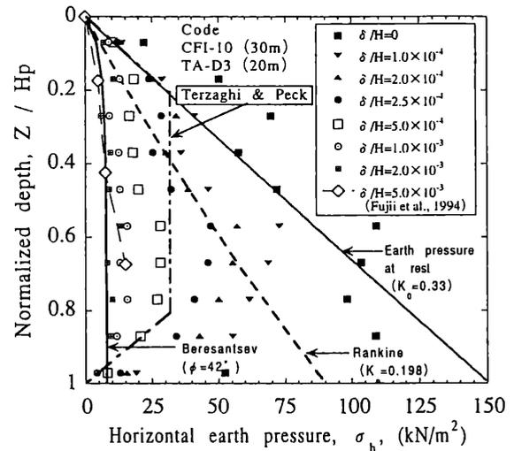
Figure 9. Active earth pressure distributions (30 m).
