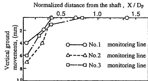
Figure 5. Ground surface settlement profiles (field data, Matsuoka et al., 1996).
