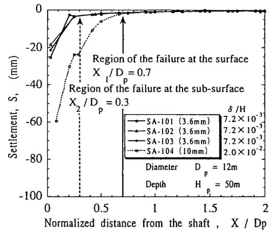
Figure 4. Ground surface settlement profiles.
