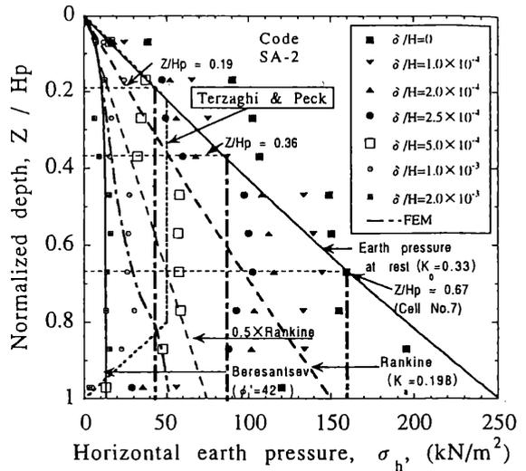
Figure 8. Active earth pressure distributions (50 m).
