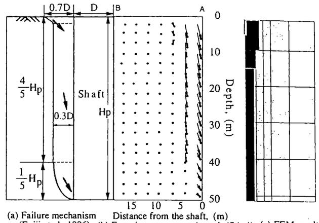
(a) Failure mechanism (Fujii et al., 1996) (b) Experiment measured result (SA-4) (c) FEM result
