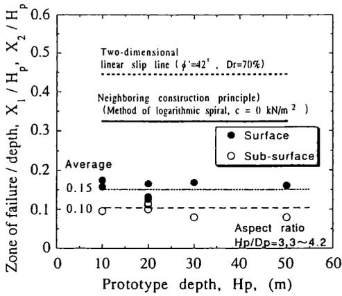
Figure 6. Relationship between the changeover depth and zone of failure normalized by  $H_p$ .
