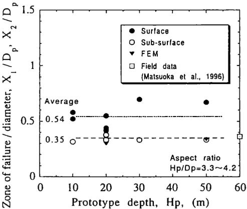
Figure 7. Relationship between the changeover depth and zone of failure normalized by  $D_p$ .
