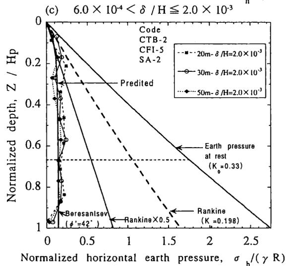
Figure 10. Predicted and active earth pressure distributions according to strain level.
