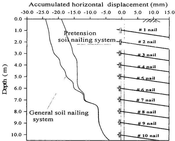
Figure 9. Comparison of accumulated horizontal displacement between pretension soil nailing system and general soil nailing system.
