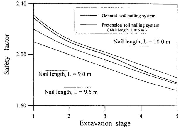
Figure 11. Comparison of nail length between pretension soil nailing system and general soil nailing system.
