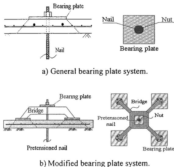
Figure 4. Schematics of the bearing plate system.
