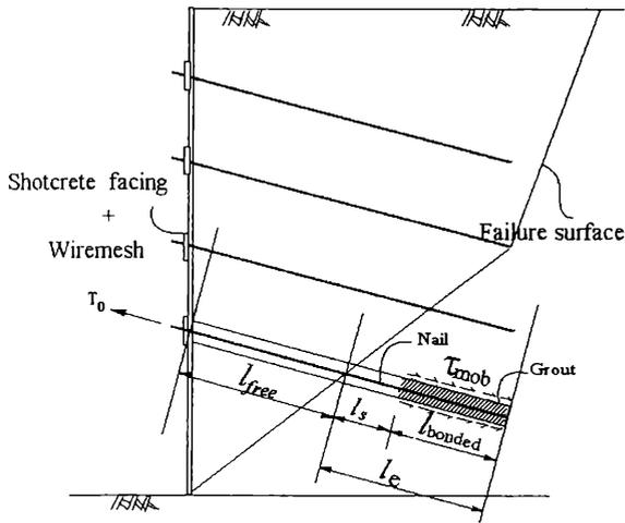
Figure 1. Description of the bonded length.
