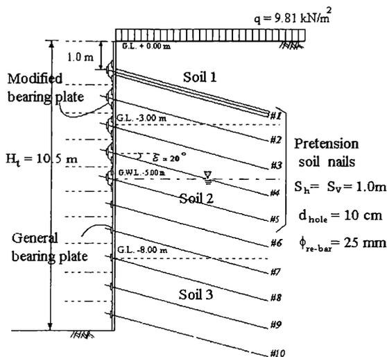
Figure 5. A cross section of the pretension soil nailing system (nail length = 9.0m).
