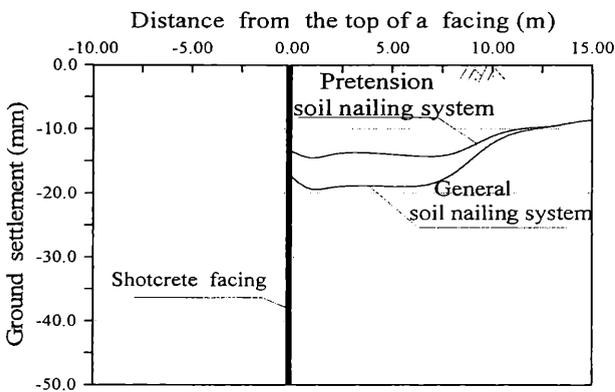
Figure 10. Comparison of ground settlement between pretension soil nailing system and general soil nailing system.
