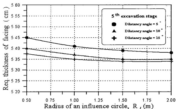
Figure 6. Relationship between radius of influence circle and required thickness of shotcrete facing.
