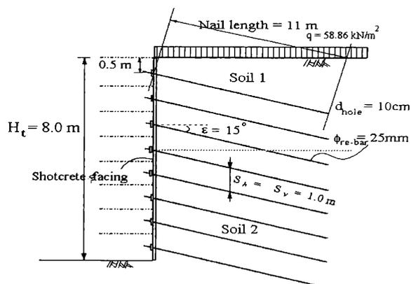
Figure 8. A cross section of the actual excavation site.
