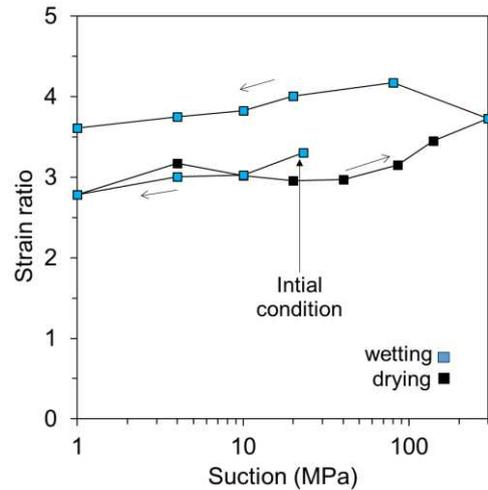
Figure 5 Ratio of the stress in the direction parallel to the direction perpendicular (stress ratio) versus the suction applied.
