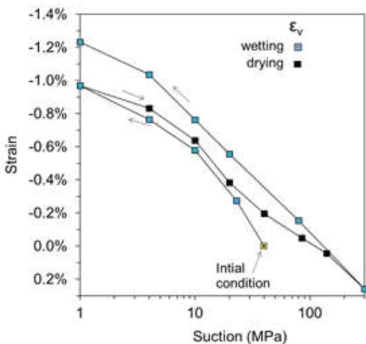
Figure 4 Volumetric strain evolution along the wetting-drying cycle.
