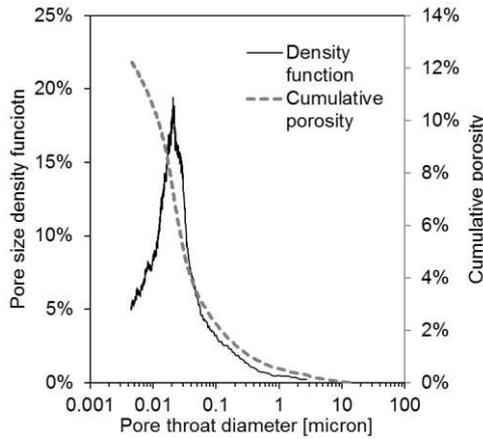
Figure 1 Pore size distribution of Opalinus Clay from 18 m depth, analysed through mercury intrusion porosimetry technique.
