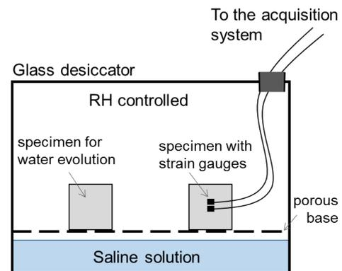
Figure 2 Simplified scheme of the adopted testing set-up: sealed glass desiccator with saline solution and tested samples.
