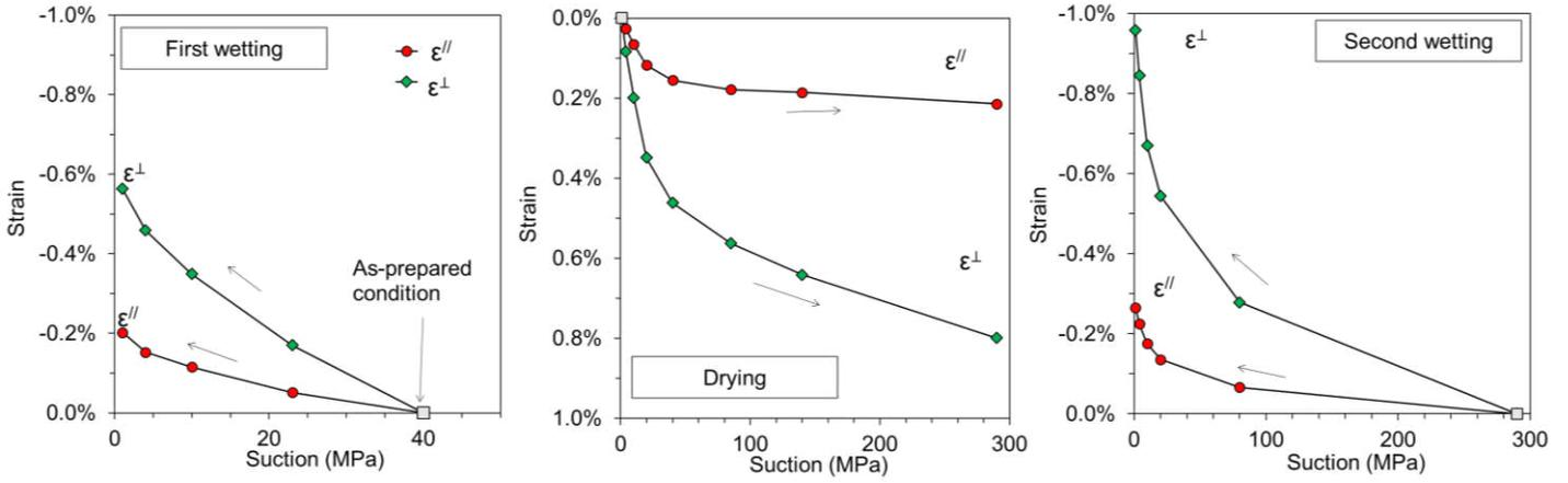
Figure 3 Strains in the direction parallel  $\epsilon^{\parallel}$  and perpendicular  $\epsilon^{\perp}$  to the bedding planes, over the suction change, depicted for first wetting, drying and second wetting phase.
