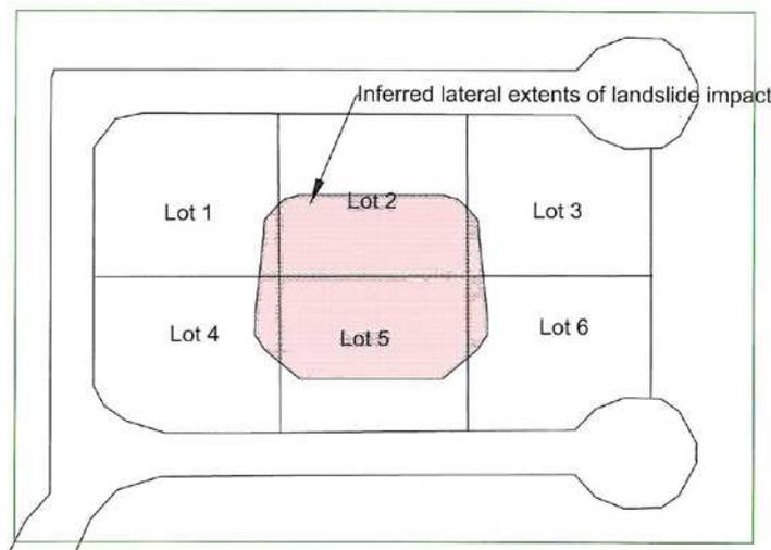
Figure 4 – Inferred aerial lateral extents of landslide
