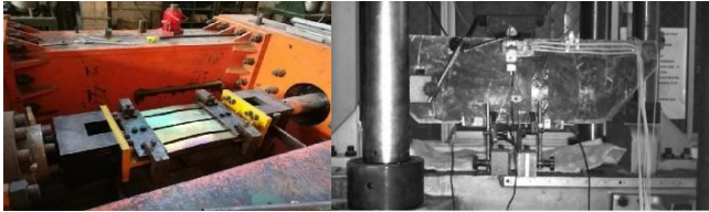
(a) SMA damping node (b) Steel fiber reinforced concrete lining Fig. 23 Methods to improve seismic resilience of shield tunnel
