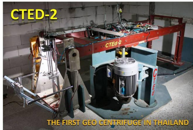
Fig. 14 The first physical-modeling centrifuge apparatus manufactured in Thailand
