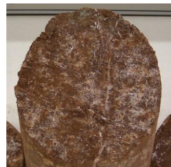
Figure 3. Gypsum crystals cover a discontinuity in anhydritic Lilla claystone
