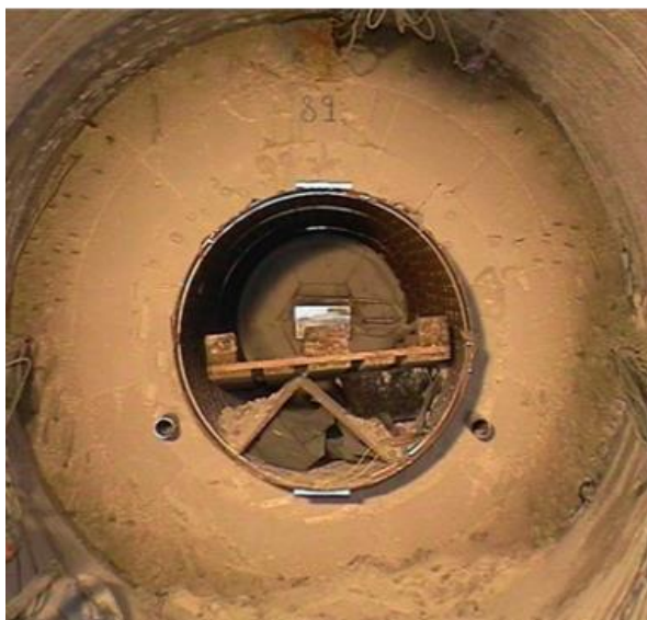
Figure 18. Bentonite barrier in large-scale Febex nuclear waste disposal test (water content and dry density) after five years of heating and hydration
