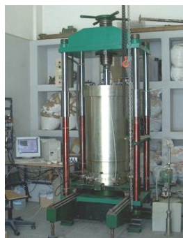
Figure 2. Relative Humidity controlled triaxial cell for rockfill aggregates
