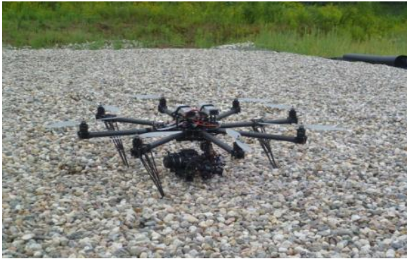
Figure 3. UAV used for monitoring wrinkles and down-slope moisture movement
