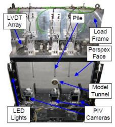
Centrifuge modelling of tunnel/pile interaction in stiff clays
