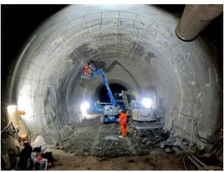
Cambridge CSIC researchers taking measurements of soil-structure interaction in newly constructed Crossrail tunnel in London using fibre optics
