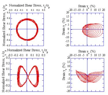
Examples of multi-directional simple shear tests on Gulf of Mexico Clay device (Rutherford, 2012)
