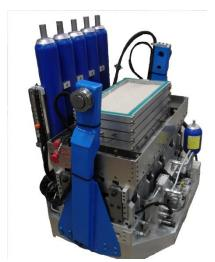
New Servo-Hydraulic Earthquake Actuator, Madabhushi et al (2012), IJPMG
