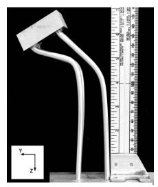
Buckling of piles in liquefied soils, Knappett & Madabhushi (2009), Geotechnique
