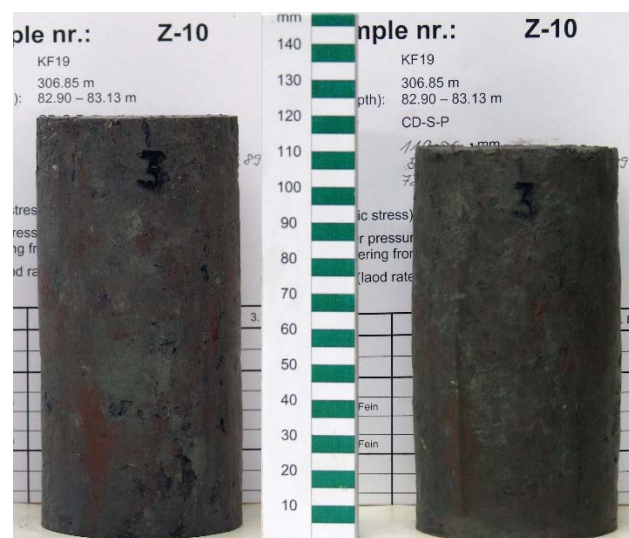
Figure 11 Breccia specimen before and after CD-testing (from Anagnostou et al. , 2012)
