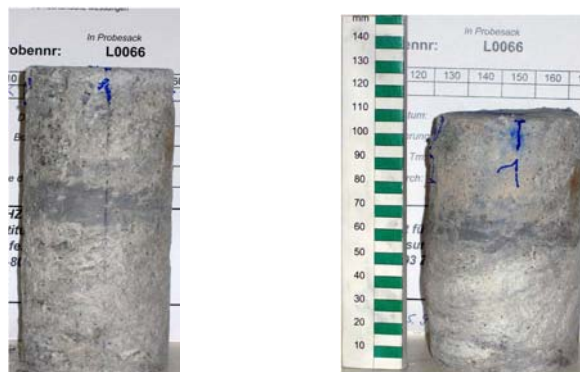
Figure 5 Kakirite specimen before and after CD-test
