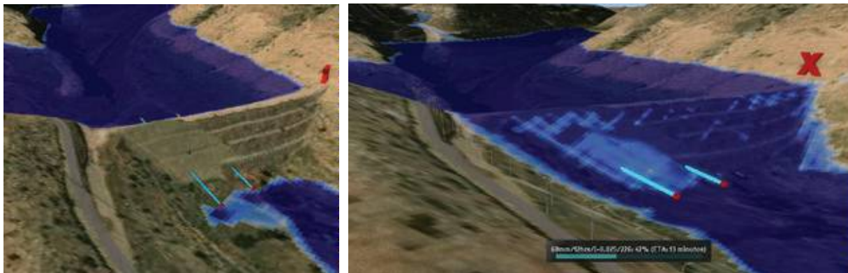
FIGURE 4.5. Screendumps of Tygron results before (left) and after the overtopping of the Abu Mansour Dam.
