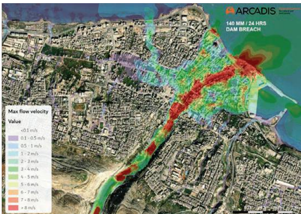
FIGURE 3.16. Maximum flow speed after the dam breach at a rainfall event of 140 mm/24 h.
