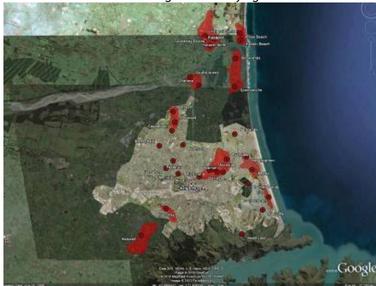
Figure 4. Areas of liquefaction (red shaded regions and red points) in Christchurch and Kaiapoi caused by the 2010 Darfield Earthquake
