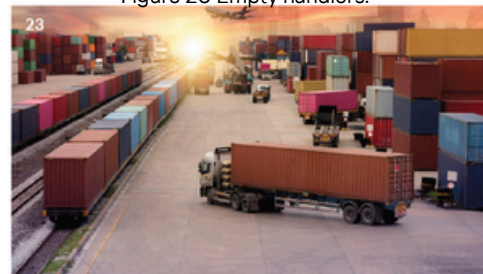
Figure 23 Internal Transfer Vehicles (ITV)
