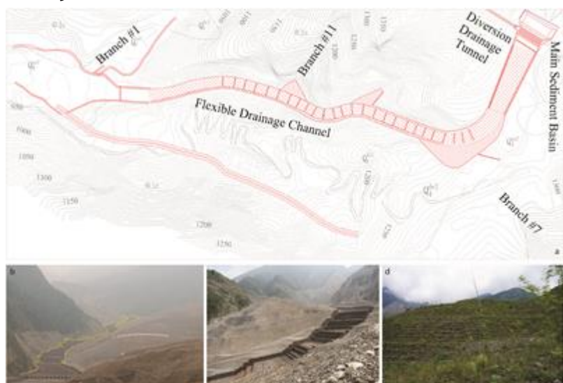
Fig. 14. The stepped flexible drainage channel in the midstream of the Wenjia Gully
