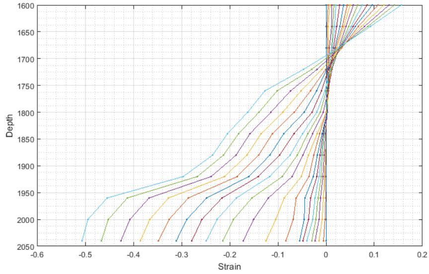
*Figure 3 - Horizontal strain distribution through clay beams at various stages of bending*
