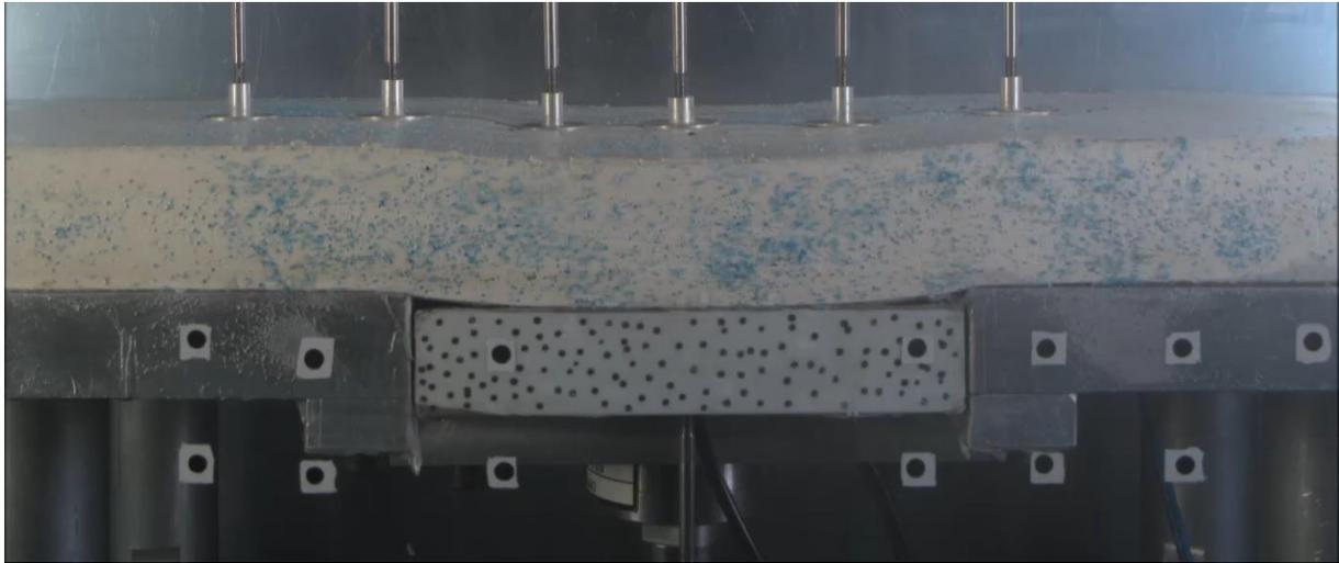
*Figure 1- Centrifuge test of clay liner over local void*
