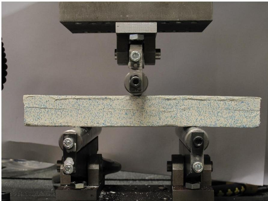
*Figure 2 - Three point bending test on clay beams*
