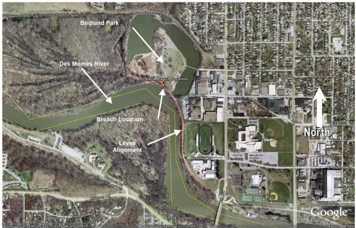
Figure 3.17 Location of the Birdland Levee breach (taken 2007).
