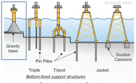
Design of gravity base foundations
