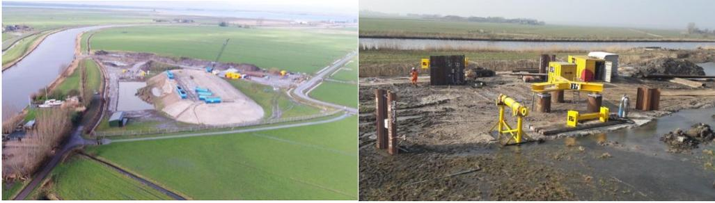
*left: Areal view of Eemdijk test, left the reference test and right the sheet pile wall test before the sheet piles were installed, right: Sheet pile push over tests*
