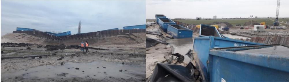
*Test view, after failure of the sheet pile wall.*
