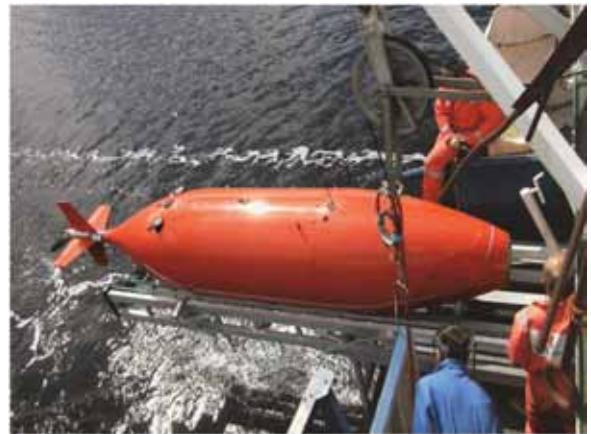
Figure 5: HUGGIN 3000 launch and recovery system (figure provided courtesy of Mr. Charlie Spann with C&C Technologies)
