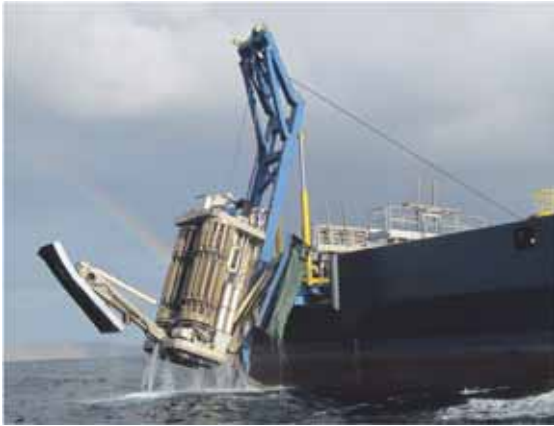
Figure 11: PROD seabed sampling and in situ testing system (figure courtesy of Mr. Alan Foley with the Benthic Group)
