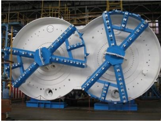
Figure 9. Double-O-Tube shield machine and concrete linings
