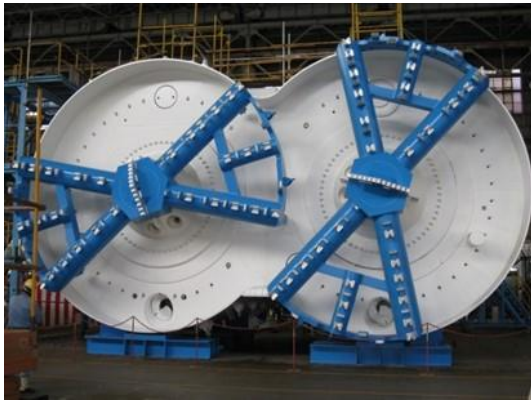
Figure 9. Double-O-Tube shield machine and concrete linings
