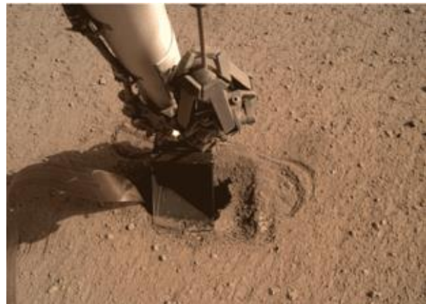
Figure 8. IDC photo showing the scoop of the Instrument Deployment Arm compressing the regolith, once the pit filled. The tether appears on the left side. The scoop width is 7.6 cm (image credit JPL/NASA).
