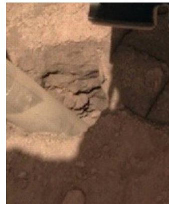
Figure 11. Image of the hole created by the HP3 mole during hammering (inclined ~15°), with the scoop appearing on top right (image credit JPL/NASA).
