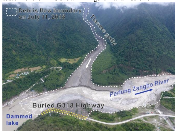
Figure 3. The Tianmo debris flow destroyed the G318 Highway in TP
