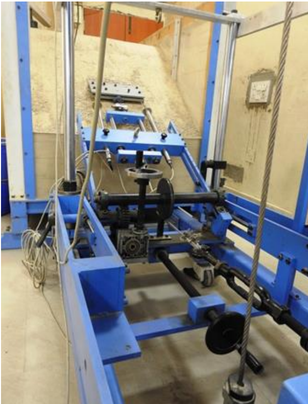
Fig. 1 The inclined pullout test set-up (Bhowmik, 2019)
