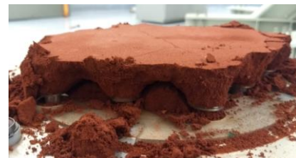
Figure 16. Soil-arching development after the B-D2H1NS test
