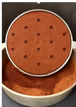
Figure 9. Typical punching failure of the D1H1NS, D1H2NS, D1H3NS tests
