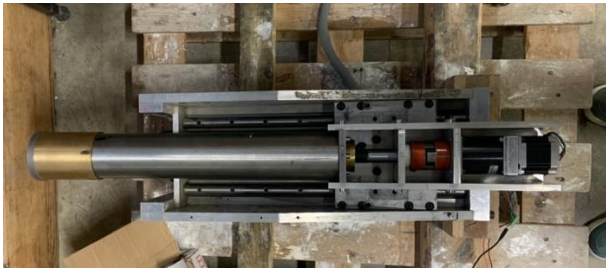
Figure 4: Photograph of the mini-TBM attached to the actuator.
