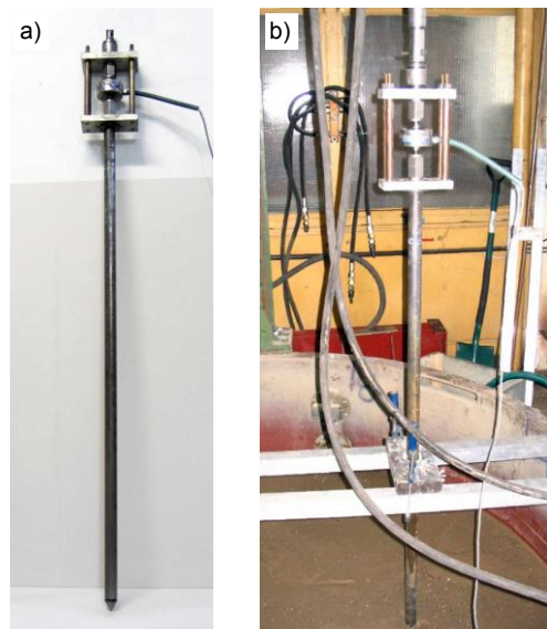
Figure 5. CPT probe design.
