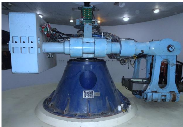
Figure 1. The TLJ-150 geotechnical centrifuge and the shaking table.
