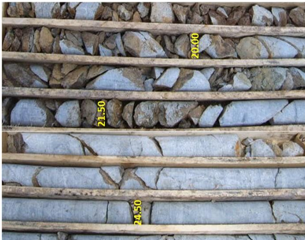
Figure 4. Core samples obtained during exploration works of Cuira Dam site, Miranda State, Venezuela.
