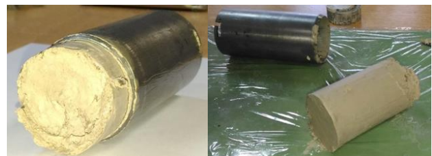
Figure 3. Specimens extracted from the two disturbed plate load tests with sampling, of the Consolidometer, intended for the preparation of the Set III of oedometer samples.
