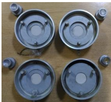
Figure 4 Oedometer samples (of Set III) made from one specimen extracted from one disturbed plate load test with sampling.
