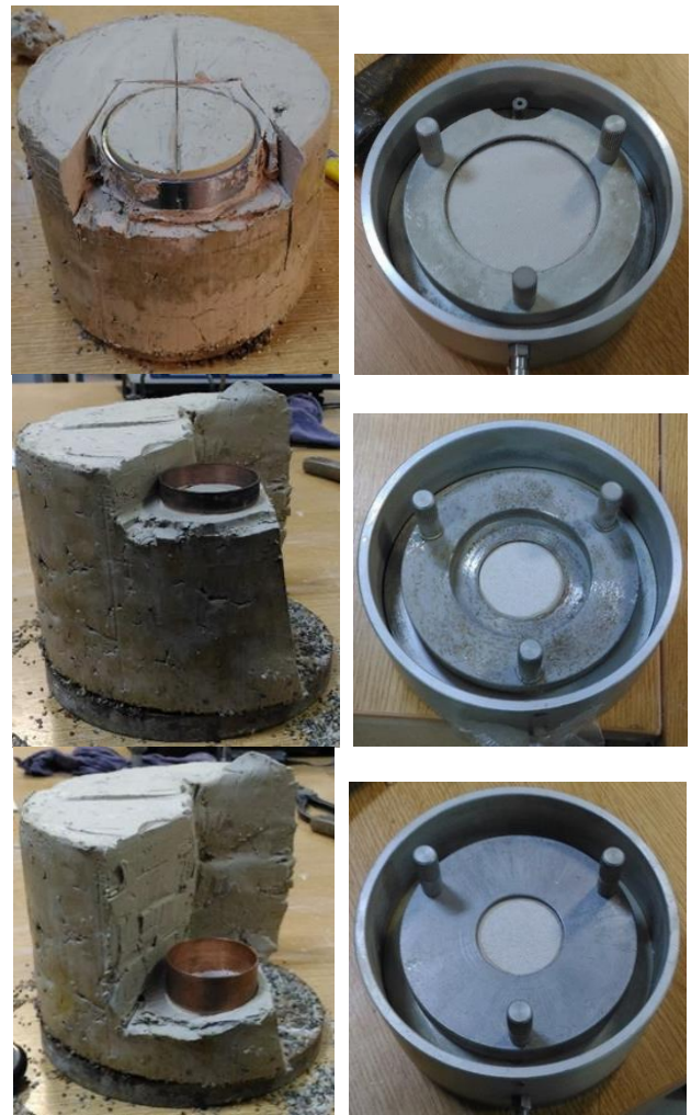
Figure 2. Preparation of oedometer samples related to Set I and II.
