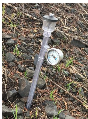
Figure 5. An installed soil suction tensiometer.
