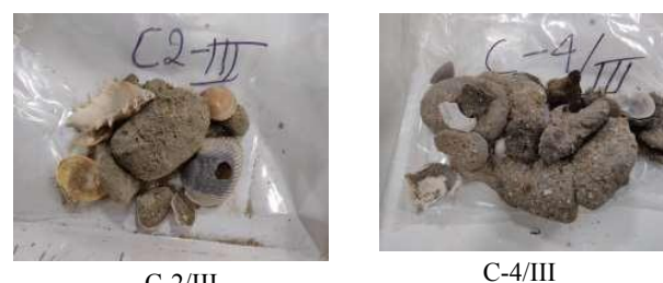
Figure 1. Pictures of lumps collected from dredged sea sand samples.
