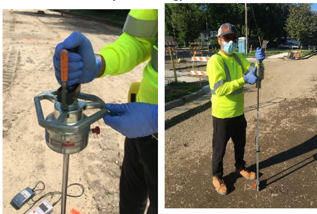
Figure 5. Light Falling Weight Deflectometer (LFWD) on top of subgrade layer, and Dynamic Cone Penetration (DCP) tests on top of the base layer
