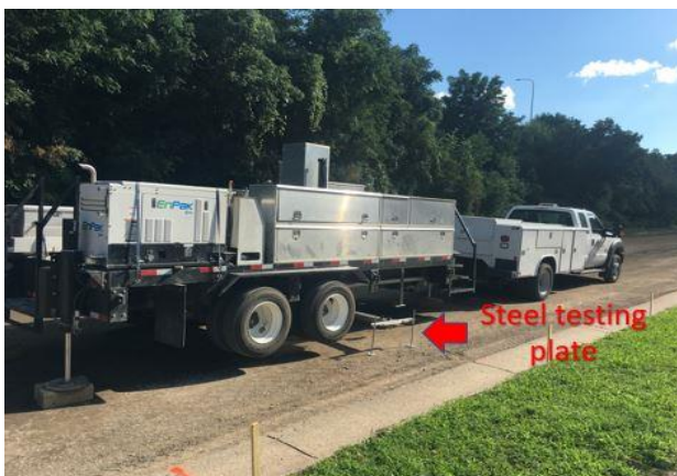
Figure 3. The Automated Plate Load Testing (APLT) system
