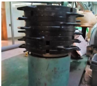
Figure 3. Reconstitution procedure: a) create a uniform slurry; b) slurry deposition in the consolidometer; c) slurry consolidation under dead-load
