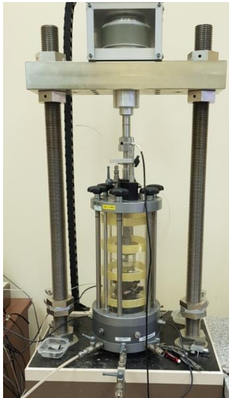
Figure 3. Triaxial compression test instrument GDS ELDYN at loading
