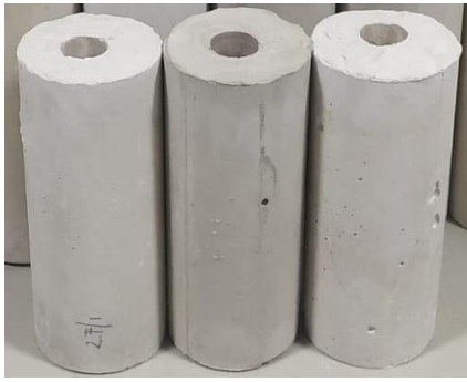
Figure 1. POP blocks prepared for the experimental program
