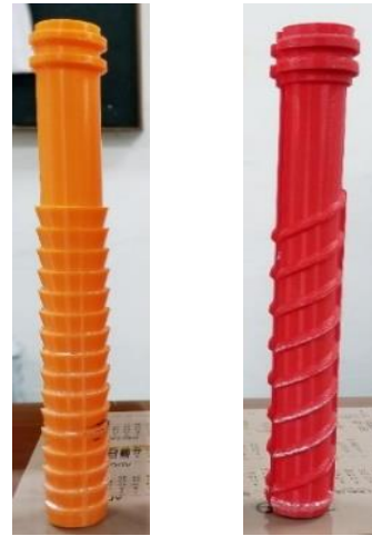
Figure 2. 3D printed Split Set models with snakeskin-inspired surface pattern and HA25 pattern
