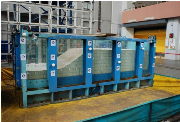
Figure 2. Layout of instrumentation including accelerometers, LVDTs, and DV in the constructed model slope and model box.
