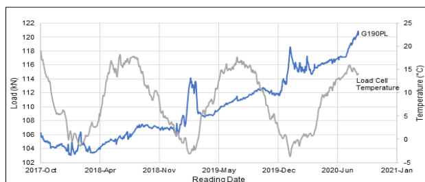
Figure 13. Load cell at the lower pile anchor compared to temperature.
